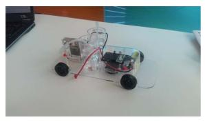
Working model of hydrogen car
